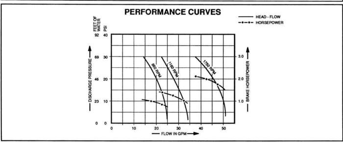
NOTE: Curve shows approximate head-flow for new pumps with neoprene impeller pumping water. Capacities should be reduced approximately 10% for nitrile, viton and EPDM impellers.
