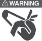
**WARNING** Injury hazard. Exposed pulleys and belts can cause injury. Install shield around pulleys and belts. Stay clear while machinery is operating.
